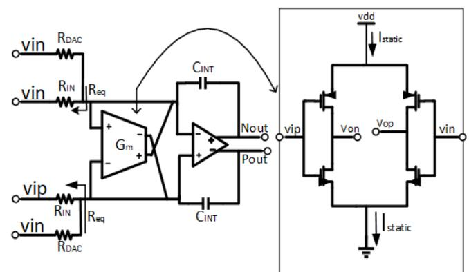
Figure 2: Negative-R Assisted Integrator
