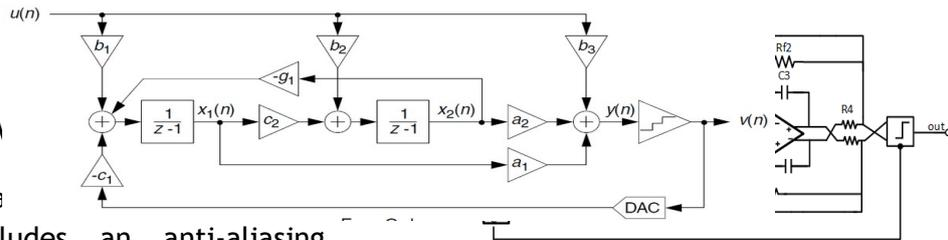
Figure 4: Block diagram of the CIFF topology
